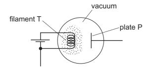
Filament T is heated and particles are emitted from it by thermionic emission.
